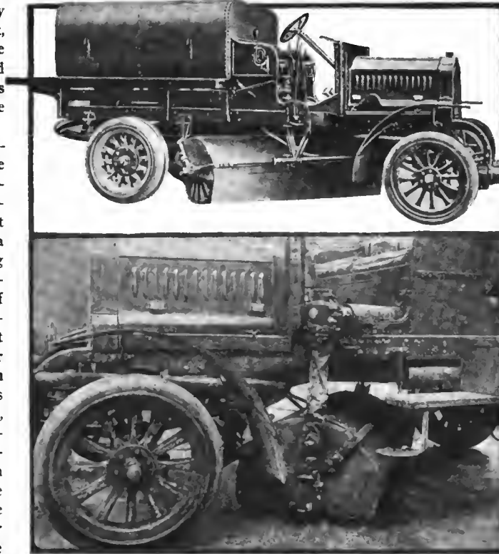
Upper—One of the rotary street sweepers in use in Paris. This is of the De Dion Bouton type. Lower—Partial side view of one of the motor-driven street sweepers, showing the driving mechanism of the rotary brush
